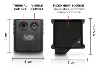
Seek Scan<sup>TM</sup> is a simple, low-cost, thermal imaging system designed to automate body temperature screening using skin temperature as a proxy. With  $\pm 0.3^{\circ}\text{C}$  ( $\pm 0.5^{\circ}\text{F}$ ) accuracy and the inclusion of a reference heat source, Seek Scan delivers the same performance as an infrared temporal thermometer – but with a safe social distance.
